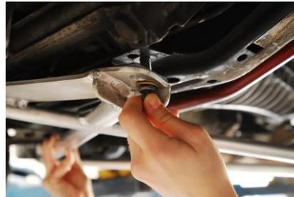
**Step 3:** Install new Allen head LCAB Bracket bolts with washers. Note: Over time, a lot of movement can occur in the uni-body, if the bracket bolts won't line up you can use a large drift punch to walk or force the brace into position.
